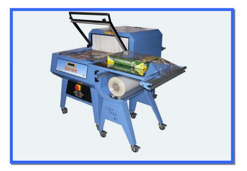
**Sealer dimensions:** 630 x 450 mm manual sealing arm Max product height: **150 mm** (extended on request) **Power supply: 380 V three phases Consumption:** 8,4 Kw **Overall machine dimensions:** 1550x1670x1120 mm Machine weight: 350 Kgs folded PO, PE and PVC Film: Max film roll dimensions: Ø 250 mm max length: 600 mm max
